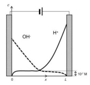
Electrolysis will split the water into H<sup>+</sup> and OH<sup>-</sup> ions. The concentration profile is shown above. At the anode, the electric field can be strong enough to split the
