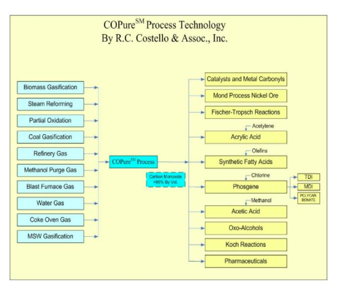
CO produced by CREDO will not be 100% pure, but this CO by-product may be commercially useful for many applications without the need for purification.
