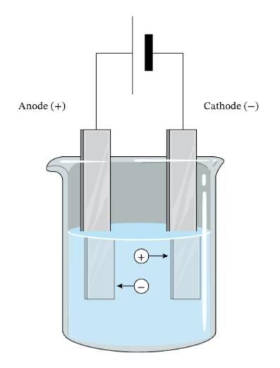
The water in our cell was tap water, with 10% dissolved baking soda (electrolyte). The vessel was filled with crushed coal with an approximate 50% coal and 50% liquid mixture. A voltage of 12 VDC and a current of 10 Amperes, dissipating a power of approximately 120 watts, was used to initiate and sustain electrolysis.
