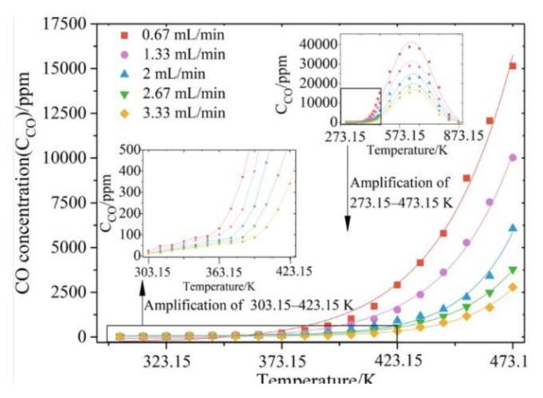
Spontaneous combustion of coal can be prevented by preventing the concentration of CO from exceeding 2000 PPM. Carbon Monoxide characteristics are described in Appendix A.
