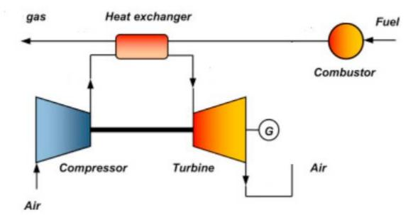
The combustor for CREDO system would be a flameless vessel and the fuel would be water and crushed coal.
