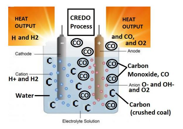
CREDO Process. Under oxygen-starvation conditions, outputs are hydrogen from the cathode and mostly carbon monoxide (CO) from the anode, and much heat at elevated temperatures. This system can be pressurized for operating at high temperature.
