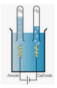
The figure above describes the most simple configuration for water electrolysis. For our experiment, the water contains 50% crushed coal (not shown) and an electrolyte, baking soda (not shown). The electrodes can be any metal.
